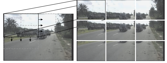
Figure 4: An example of dividing an image up in overlapping regions. In this particular example, the region size is a \frac{1}{2} of the image size for both the x-dimension and y-dimension. The regions are uniformly sampled across the image with a step size of half a region. Sampling in this manner identifies nine overlapping regions.
