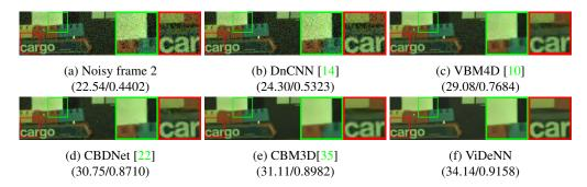
Figure 9: Detailed comparison of denoising algorithms on the low-light video *Train* with light intensity at 50/255. Our ViDeNN shows good performance in this light condition, preserving edges and correctly smoothing flat areas. Results referred to frame 2, expressed in terms of (PSNR [dB]/SSIM).
