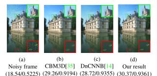
Figure 3: Comparison of spatial denoising of an image from the CBSD68 dataset corrupted with 1, with Ag=64 and Dg=4. AWGN based method as CBM3D and DnCNN does not achieve optimal result. The first blurs excessively the image. Using the proper noise model for training leads to a better result. (PSNR [dB]/SSIM)
