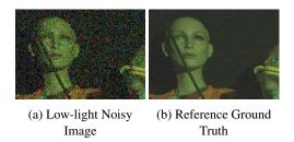
Figure 4: Sample detail of noisy-clean image pairs of our own low-light dataset, collected with a Bosch Autodome IP 5000 IR security camera. The ground truth is obtained averaging 200 raw images collected in the same light conditions.
