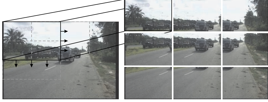
Figure 3.3: An example of dividing an image up in overlapping regions. Here, the region size is a \frac{1}{2} of the image size for both the x- and y-dimension. The regions are uniformly sampled across the image with a step size of half a region. Sampling in this manner identifies nine overlapping regions.
